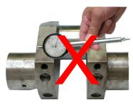
Most engineers know the importance of regularly checking the rectilinear of the crankshaft on marine diesels. The usage of an indicator clock was timeconsuming, unpleasant, dirty and yielded dubious measurement results. As a consequence these checks were made less
